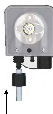
Screw the clear pipe on the metering pump...
